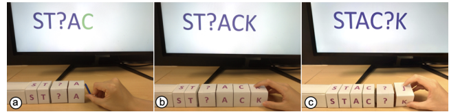
Figure 10: Stacking of boxes on an adapter stacked on a station: (a) sensing other NFC tags, (b) without rotation, and (c) with rotation.
