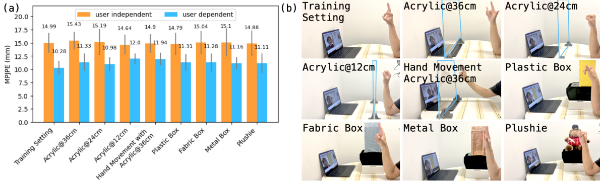
Fig. 11. Ring-a-Pose’s Robustness to Nearby Surfaces and Objects. (a) Using models trained with data collected in the same setting, the testing results on data collected in various settings show Ring-a-Pose’s performance with nearby surfaces and objects. (b) Training and Tested Settings. The acrylic sheets are highlighted in light blue. Error bars in this figure represent the standard deviation.
